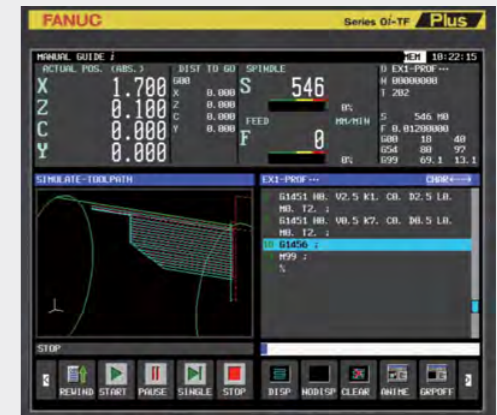
Check cutting path using cutting simulation
