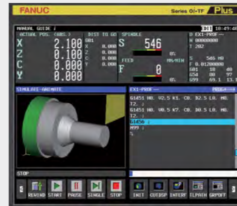
Check cutting result using cutting simulation
