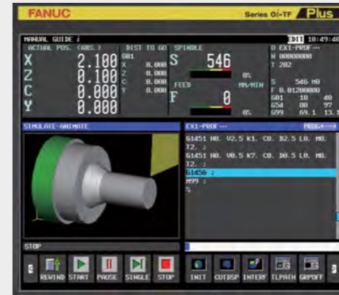
Check cutting result using cutting simulation
