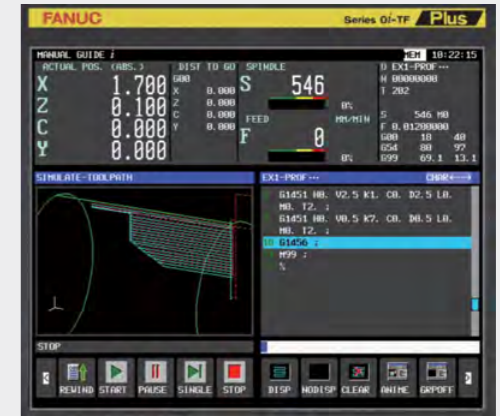
Check cutting path using cutting simulation
